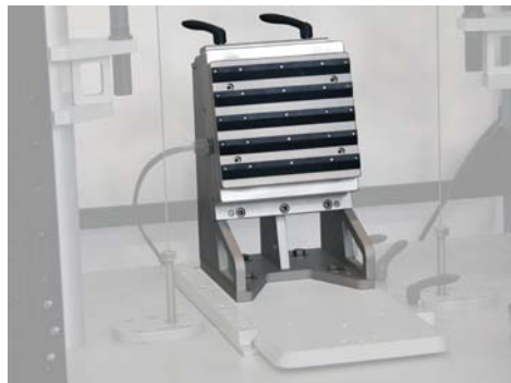
Instrumented anvil with load cells for tangential force reading
